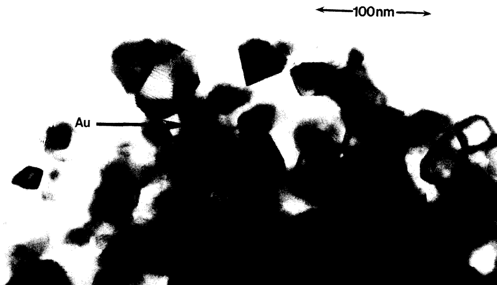
FIG. 11. TEM picture of Au/TiO 2 heated to 700°C.
