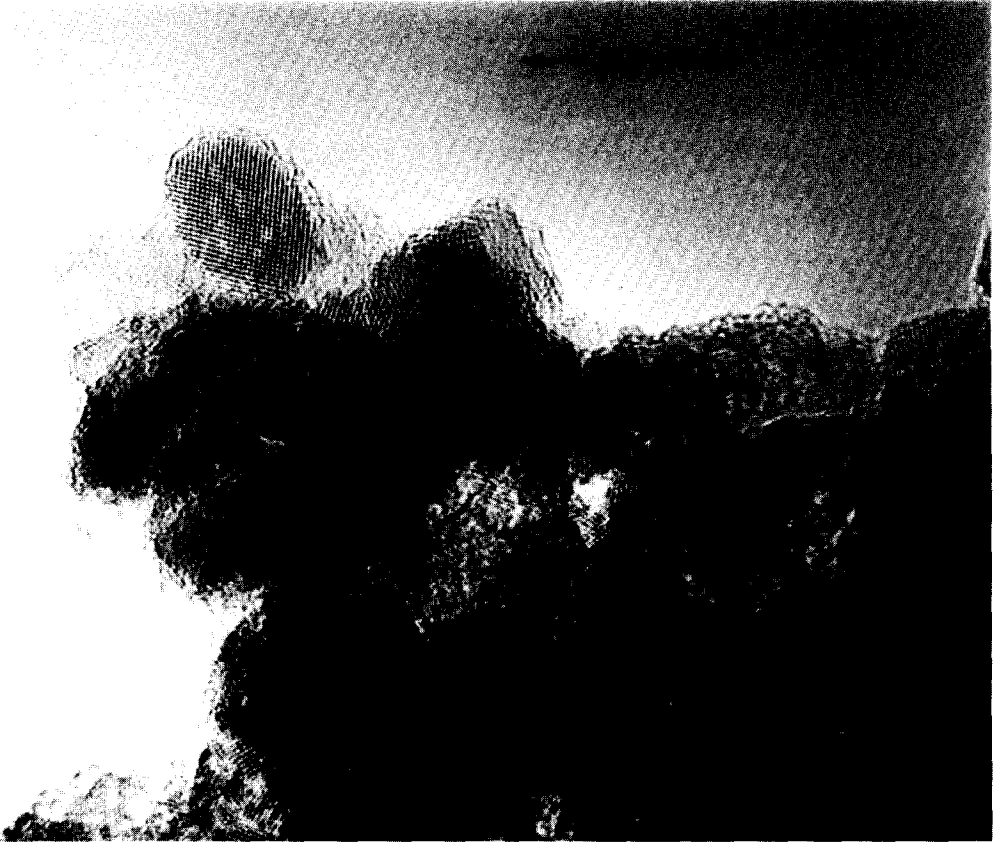
FIG. 7. High-resolution transmission electron micrograph of Au/TiO 2 (fresh sample).
